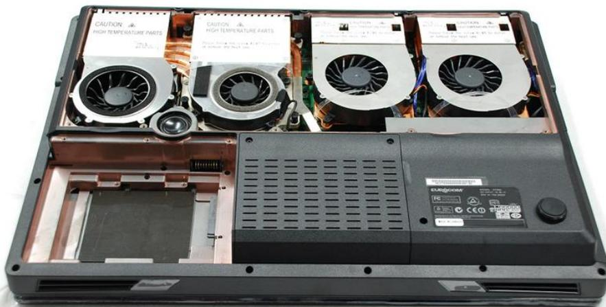
*The code-name "Copper Mountain" would have been suitable for Eurocom's Panther server system. With a heatsink-fan mounted over the CPU, chipset, and both GPUs, the unit stays remarkably cool even under sustained load.*
